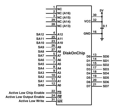
Figure 1: DiskOnChip Pins
